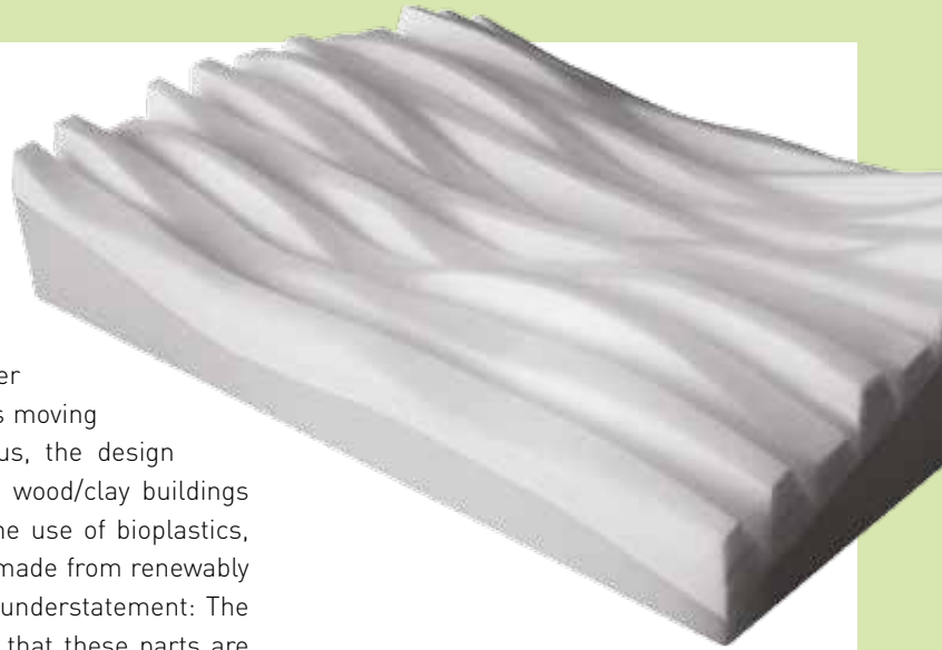
Paneling, thermoformed bioplastic-example by research group: itke, iswa, Tecnaró, Bauer, spek Design (Foto: spek Design)
